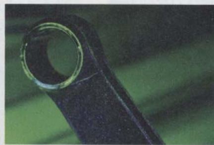
↑ This is a photo of the cracked connecting rod that engine builder Keith Dorton used as an example in his discussion on finding the true reason for part failures in order to build better racing engines.
